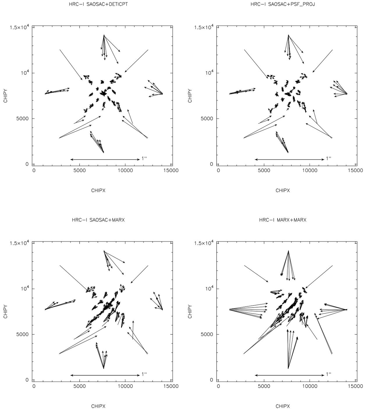
**Figure 3.** Individual bright point source observations: vector diagrams representing the shift from centroids of the observed detections to centroids of the simulated rays. Positional offsets are scaled by a factor of 1000 to exaggerate the deviations. The arrow at the bottom denotes shifts of 1'' ( $\sim 7.5$  HRC pixels) in this scaling convention. Quantitative analysis of these offsets is shown in Table 1.
