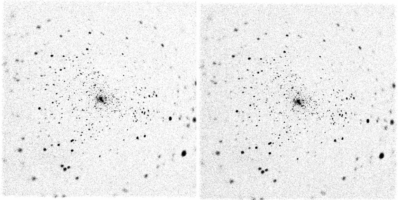
**Figure 1.** LEFT: The Orion Nebular Cluster on HRC-I, in SKY coordinates, as determined by standard pipeline processing. RIGHT: ONC on HRC-I in CHIP coordinates, after telescope dither is manually removed.
