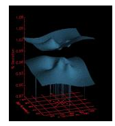
This plot shows the error on the gain correction map as percentage deviations. Errors are derived from matching the shapes of the PHA distributions as shown in Panel 6. The surface is determined as the minimum curvature surface for the 3–sigma deviations from the best-fit correction to the gain correction map. The circles indicate the locations of the AR Lac pointings.
