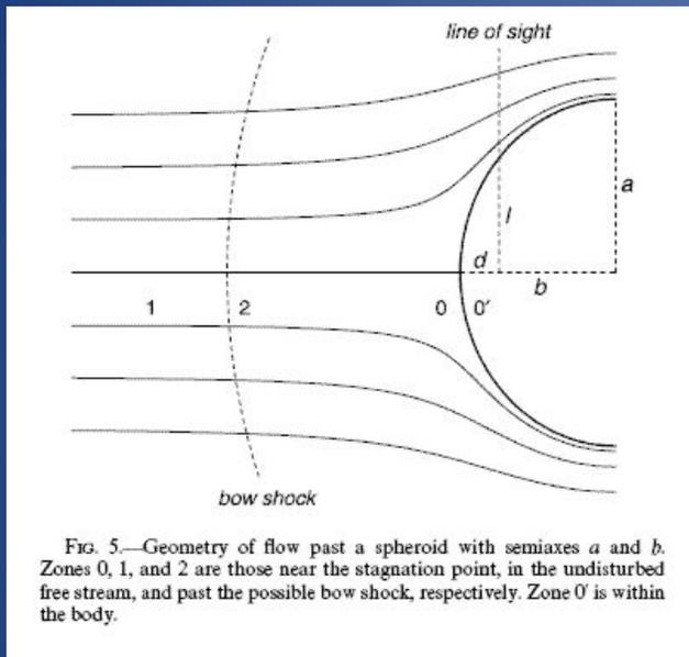
FIG. 5.—Geometry of flow past a spheroid with semi-axes  $a$  and  $b$ . Zones 0, 1, and 2 are those near the stagnation point, in the undisturbed free stream, and past the possible bow shock, respectively. Zone  $O'$  is within the body.
