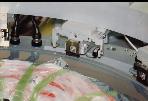
The success of the HRMA alignment and the ultimate performance of the observatory is linked to the high fidelity process development enabled by the VETA-II "build" with aluminum mirror simulators and the real uncoated P1/H1 mirrors. The mirror bonding process was initially unsuccessful and would have led to unacceptable system performance without the VETA-II.
