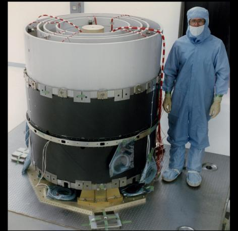
VETA-II with P1/H1 aluminum mirror simulators removed. Ready for tower alignment demonstration
