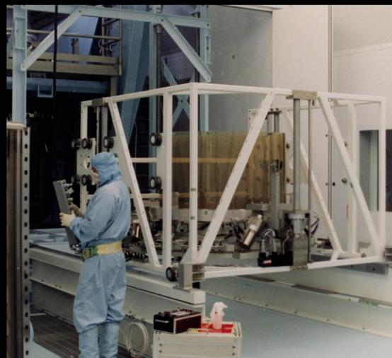
H1 simulator moving into position for the VETA-II handling demonstration
