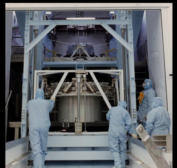
Close-up of MAS offloader on H1 mirror
