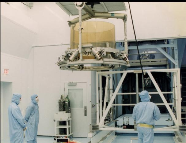
Uncoated P1 mirror on parts carriage for installation onto VETA-II
