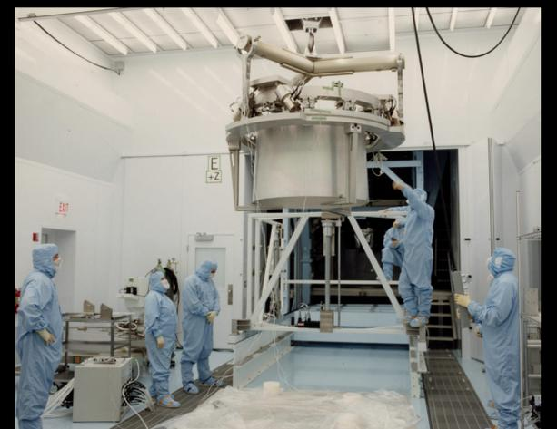
Uncoated P1 mirror moving into alignment tower on MAS
