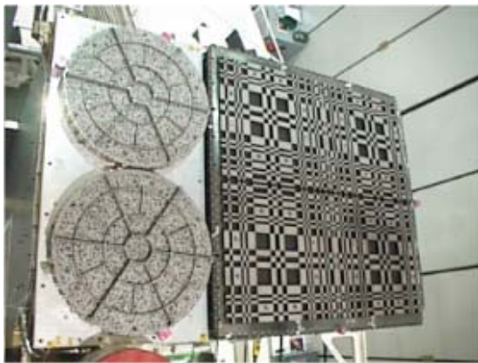
Coded Aperture Optics: high background, large detector
