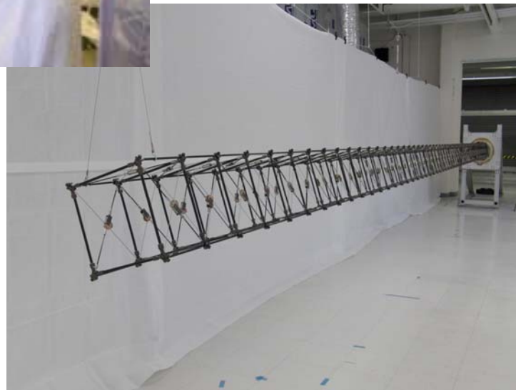
ATK/Goleta: extendable mast fully deployed flight mast
