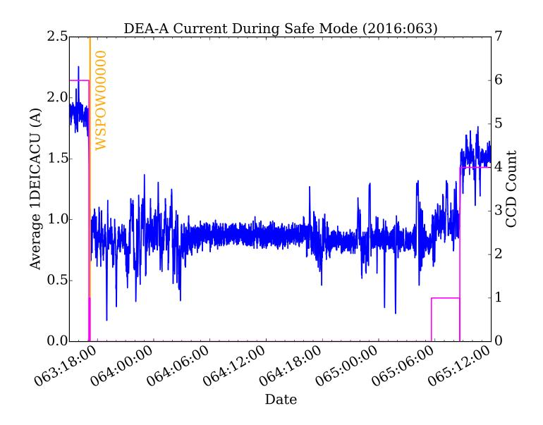
Figure 2: Average behavior of 1DEICACU during a safe mode. All video boards are powered off after the issuing of the WSPOW00000 command, which is marked by the orange line in the plot.
