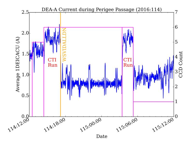
Figure 1: Average behavior of 1DEICACU during a perigee passage. All video boards are powered off after the issuing of the WSVIDALLDN command, which is marked by the orange line in the plot.
