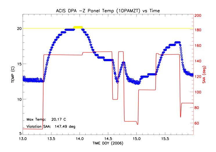
Figure A.4: Plot of temperature versus time for a 1DPAMZT yellow high limit trip on day 13 of 2006. Included in red on this plot is the SAA for the duration of the trip. Notice the extremely sensitive dependence of this thermistor to a small change in SAA.
