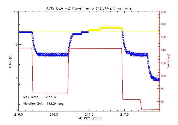
Figure A.1: Plot of temperature versus time for 1DEAMZT during a yellow high limit trip on day 216 of 2005. Included in red on this plot is the SAA for the duration of the trip. The duration listed on the plot is the total time that 1DEAMZT spent above the yellow limit regardless of temperature fluctuations above this level.
