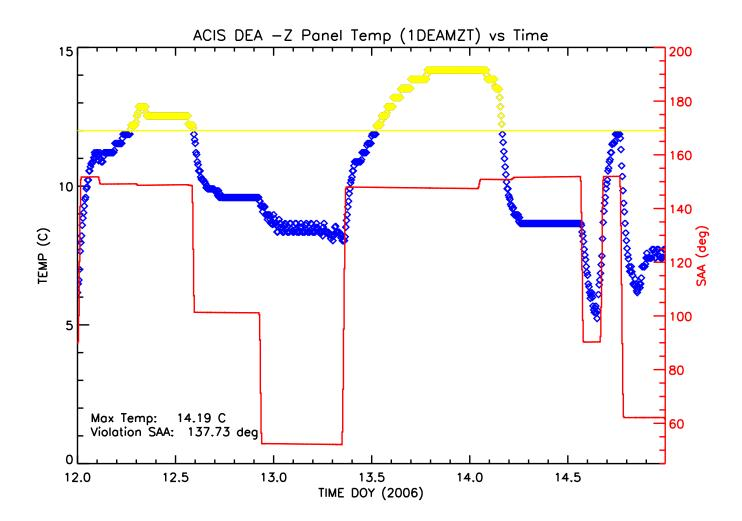
Figure A.3: Plot of temperature versus time for 1DEAMZT during a yellow high limit trip on days 12 and 13 of 2006. Included in red on this plot is the SAA for the duration of the trip. The duration listed on the plot is the total time that 1PIN1AT spent above the yellow limit regardless of temperature fluctuations above this level.
