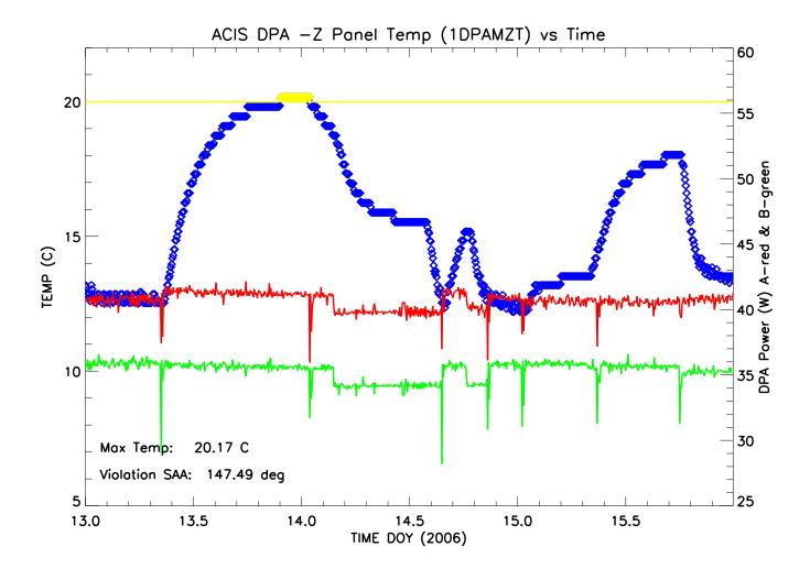
Figure A.5: Another plot of temperature versus time for 1DPAMZT during a yellow high limit trip on day 13 of 2006. Included in red and green on this plot is the DPA power consumption. The slight drop in power after the trip is indicative of commanding the ACIS CCDs for a calibration observation while entering perigee.
