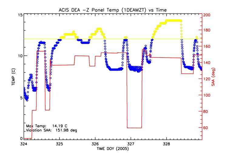
Figure A.2: Plot of temperature versus time for 1DEAMZT yellow high limit trip on days 324-328 of 2005. Included in red on this plot is the SAA for the duration of the trip. The duration listed on the plot is the total time spent above the yellow limit regardless of temperature fluctuations above this level.
