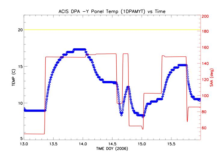
Figure A.6: Plot of temperature versus time for a 1DPAMYT during the 1DPAMZT yellow high limit trip on day 13 of 2006. Included in red on this plot is the SAA for the duration of the trip. Notice the extremely sensitive dependence of this thermistor to a small change in SAA.
