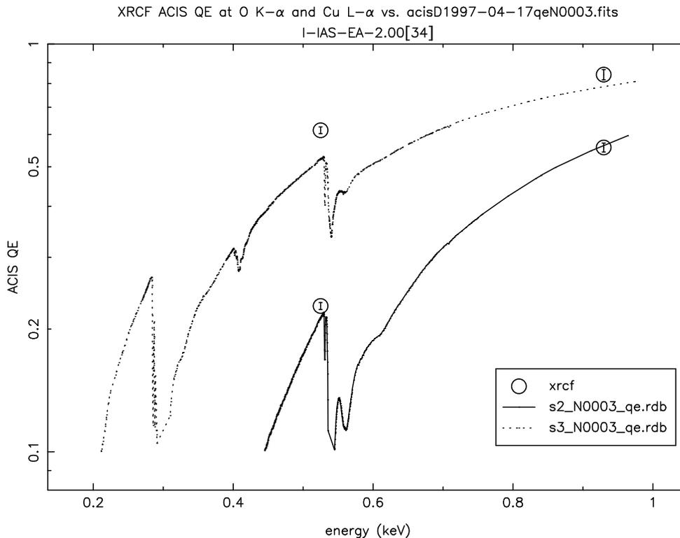
Figure 5: Derived QE of S3 and S2 at oxygen K- $\alpha$  and copper L- $\alpha$ . Also plotted are the released CALDB products from file `acisD1997_04_17qeN0003.fits`
