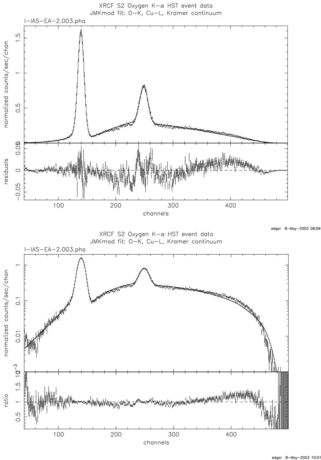
Figure 1: JMKmod fit to full-chip S2 data from I-IAS-EA-2.003
