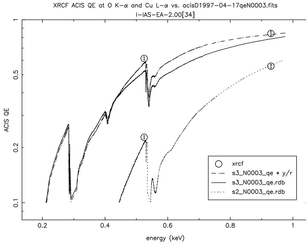
Figure 6: Derived QE of S3 and S2 at oxygen K- $\alpha$  and copper L- $\alpha$ . Also plotted are the released CALDB products from file `acisD1997_04_17qeN0003.fits`, and the corrected S3 quantum efficiency curve,  $y/r QE_{S3}$ . The correction factors are  $r$ , Marshall's empirical grating correction, and  $y$ , the flight FI decrement due to cosmic ray dead area (see text).
