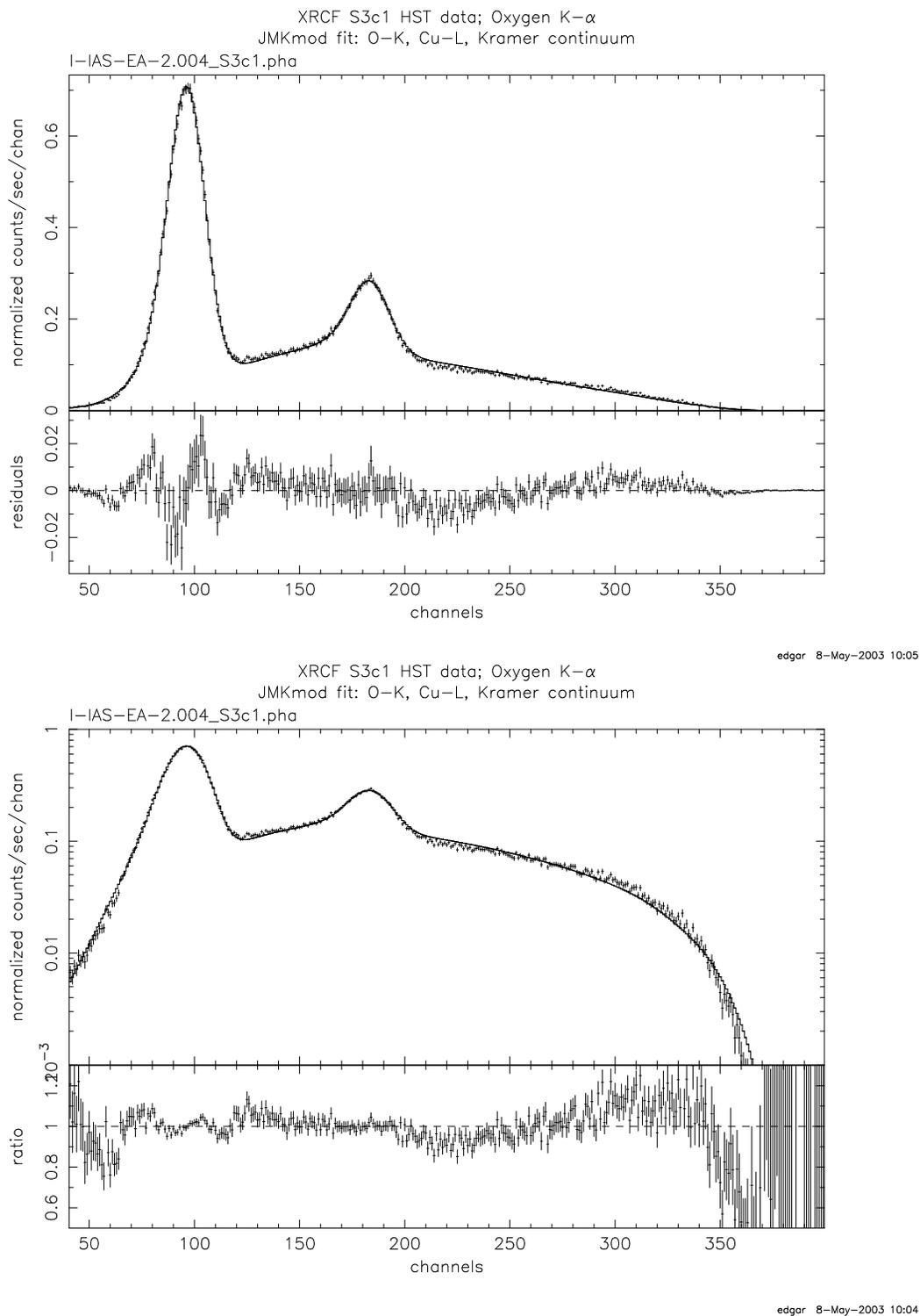
Figure 3: JMKmod fit to single-node S3c1 data from I-IAS-EA-2.004
