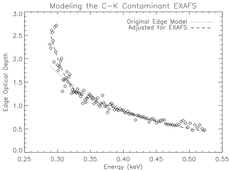
**Figure 5.** Similar to the bottom half of Fig. 4 except the data have been rebinned to reduce statistical noise and only the region being fit for extended fine structure is shown. The Henke model of the C-K edge (short dashed line) is a good match to the data in the 0.38 to 0.48 keV range, so the Henke optical constants are used above 0.48 keV. Below 0.38 and down to the edge, a damped oscillation adjustment is used (eq. 2).
