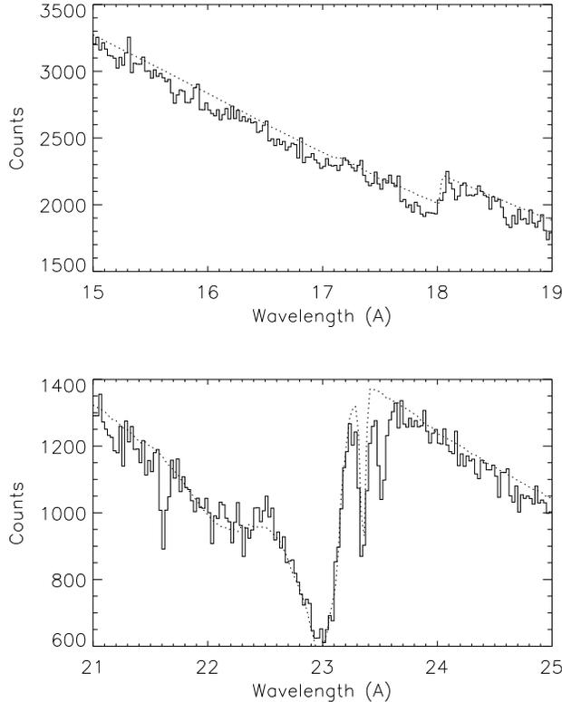
**Figure 8.** Count spectra at the edges of F-K (top) and O-K (bottom). The overall structure is modeled to better than 3% and the only remaining features are intrinsic to the source (or to the gas between the target and the telescope, see Nicastro et al. 2003, in preparation). There is a slight normalization error in the F-K edge region due to the systematic effects of correcting for the relative error in the BI QEs compared to the FI QEs.<sup>4</sup>
