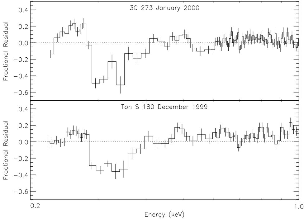
**Figure 1.** Comparison of two LETG/ACIS-S observations of bright continuum sources. The residuals give the fractional differences between the simple power law spectral model that was folded through the instrument response and the observed count spectra. Note the apparent edge at about 0.29 keV, which is near the K edge of carbon. The data were adaptively binned to obtain a signal to noise ratio of at least 20 in each bin, limited to a bin width  $< 5\%E$  at energy  $E$ .
