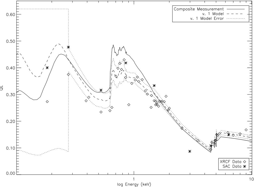
the “out of band” response of the detector. We have chosen a balanced approach and modified both the low energy and “out of band” response models. This results in comparatively greater uncertainties for the response at low energies, which we estimate to be 20% below 277 eV. While still large, this is a significant improvement over the low energy uncertainties in the original flight model. All of these uncertainties are at the one sigma confidence level.
