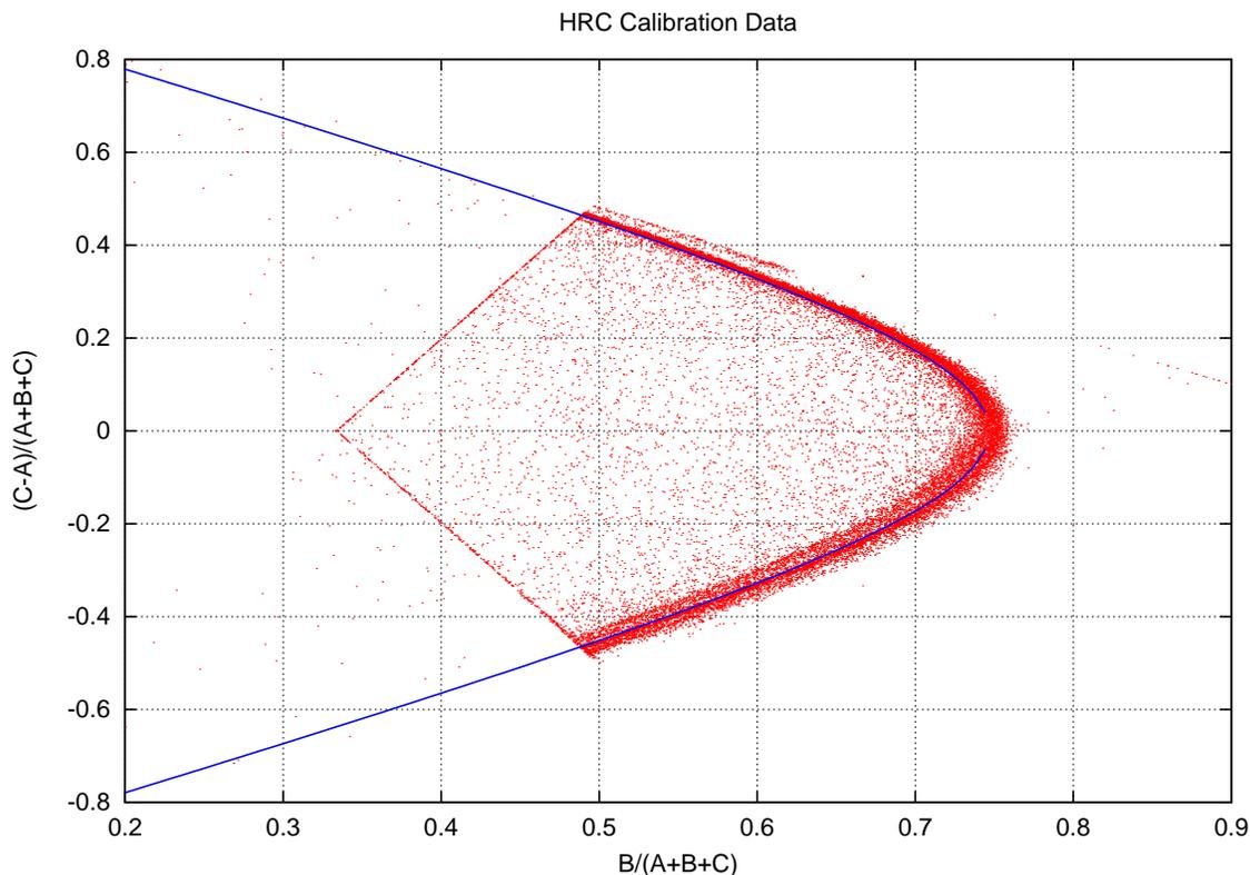
Figure 5: An  $f_p, f_b$  plot for the HRC-I from data obtained during on-orbit calibration source observation. Also shown is the best fit hyperbolic function for these data, using the parameters listed in Table 1
