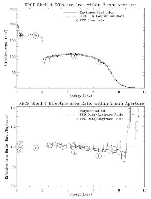
Figure 11.38: Calibration data vs. raytrace prediction. Top panel shows the XRCF Shell 4 effective area within 2 mm aperture. Bottom panel shows the effective area ratio of data/raytrace.
