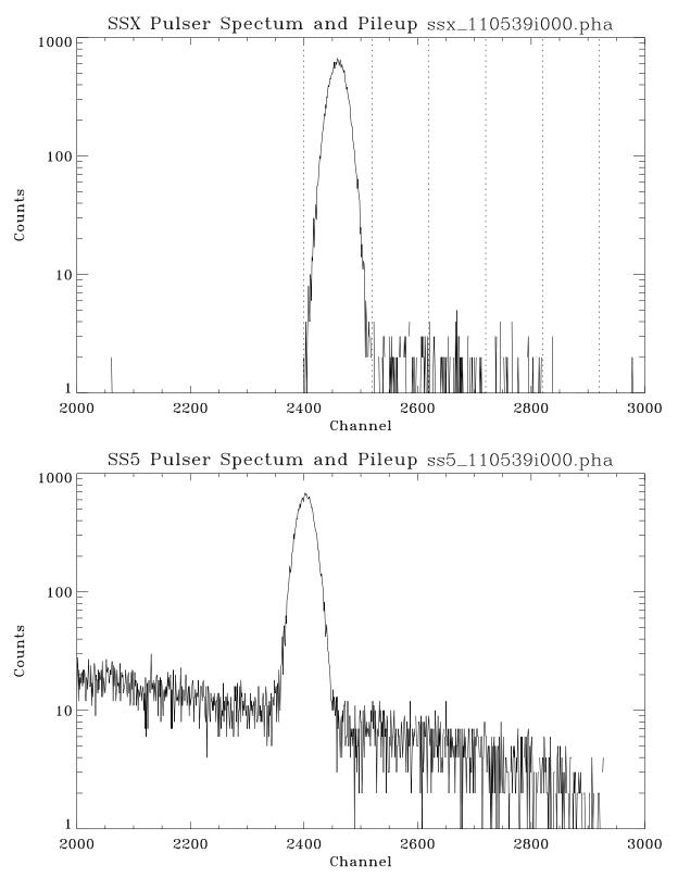
Figure 11.5: SSX and SS5 pulser spectra: Shell 1; Run ID: 110539. Counts to the right of the SSX pulser peak are the pileups from the pulser and low energy photons. Dotted vertical lines in the upper panel indicate the pulser region and four pileup bands.
