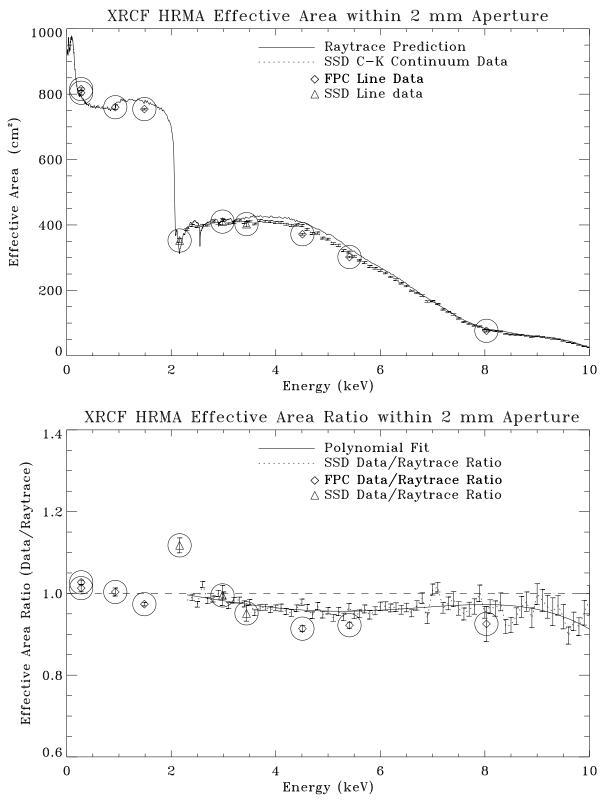
Figure 11.40: Calibration data vs. raytrace prediction. Top panel shows the XRCF HRMA effective area within 2 mm aperture. Bottom panel shows the effective area ratio of data/raytrace.
