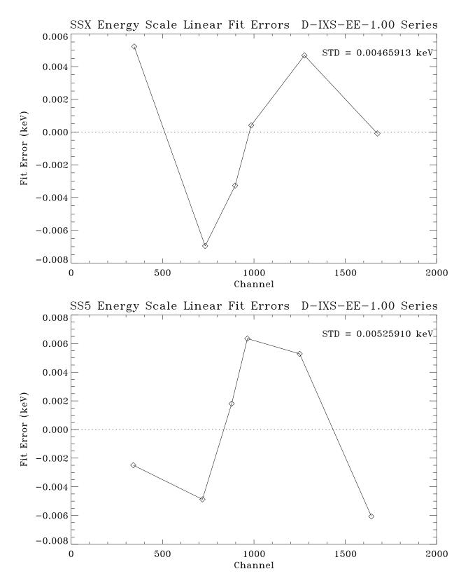
Figure 11.24: SSX and SS5 energy scale linear fit residuals for the C-continuum effective area measurements (Phase-D).
