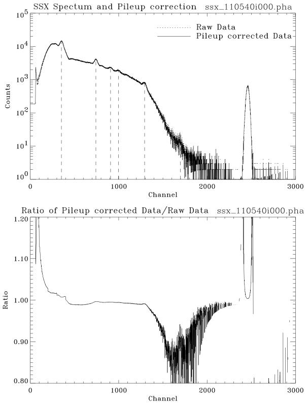
Figure 11.10: SSX spectrum and pileup correction: Shell 3; Run ID: 110540. Upper panel shows the raw data and pileup corrected data. Dashed vertical lines indicate the X-ray lines to be used to calibrate the energy scale. Lower panel shows the ratio of pileup corrected data to the raw data.
