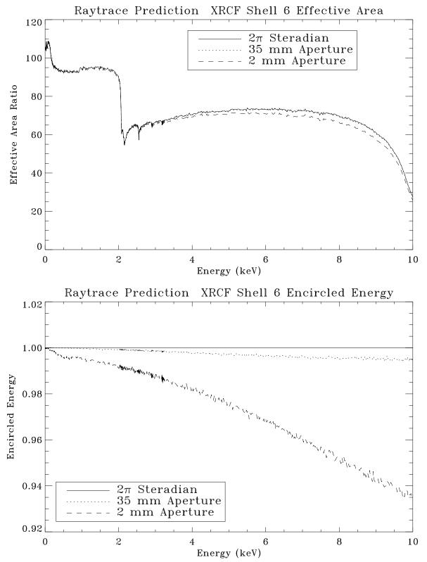
Figure 11.44: Ray trace prediction of XRCF Shell 6 effective area and encircled energy. Top panel shows the effective area curves within 2 mm, 35 mm apertures, and  $2\pi$  steradian. Bottom panel shows the encircled energies of 2 mm and 35 mm apertures as fractions of that within  $2\pi$  steradian.
