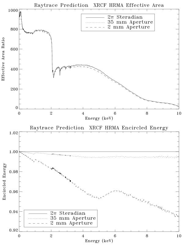
Figure 11.45: Raytrace prediction of XRCF HRMA effective area and encircled energy. Top panel shows the effective area curves within 2 mm, 35 mm apertures, and  $2\pi$  steradian. Bottom panel shows the encircled energies of 2 mm and 35 mm apertures as fractions of that within  $2\pi$  steradian.
