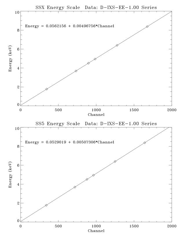
Figure 11.23: SSX and SS5 energy scales for the C-continuum effective area measurements (Phase-D), fitted with six X-ray line energies, averaged over four spectra (Run IDs: 108426, 108450, 108484, 108500).
