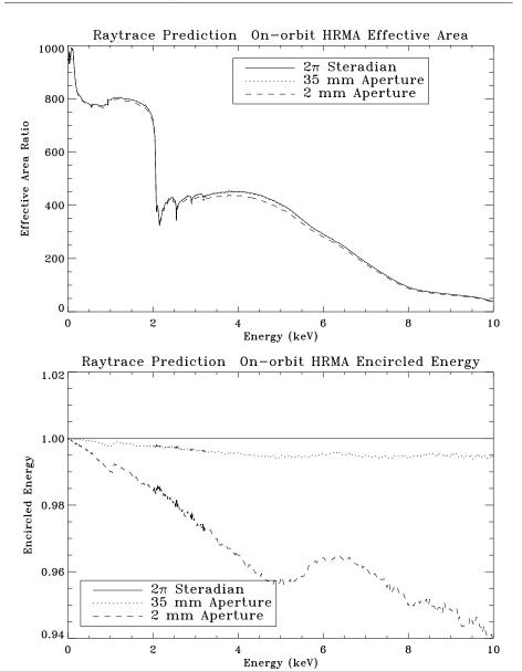
Figure 11.50: Raytrace prediction of on-orbit HRMA effective area and encircled energy. Top panel shows the effective area curves within 2 mm, 35 mm apertures, and  $2\pi$  steradian. Bottom panel shows the encircled energies of 2 mm and 35 mm apertures as fractions of that within  $2\pi$  steradian.
