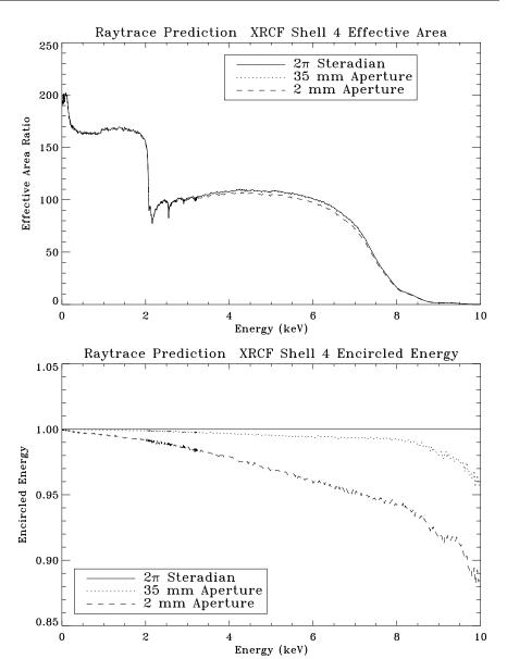
Figure 11.43: Ray trace prediction of XRCF Shell 4 effective area and encircled energy. Top panel shows the effective area curves within 2 mm, 35 mm apertures, and  $2\pi$  steradian. Bottom panel shows the encircled energies of 2 mm and 35 mm apertures as fractions of that within  $2\pi$  steradian.
