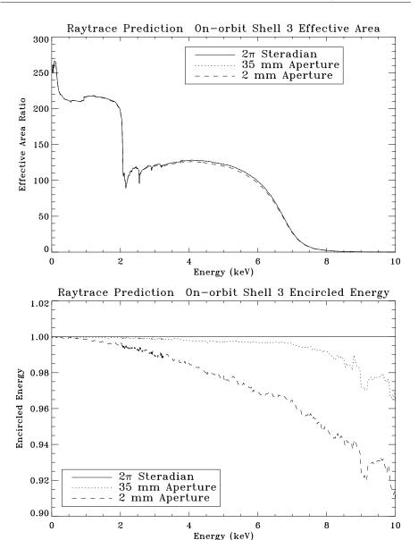
Figure 11.47: Ray trace prediction of on-orbit Shell 3 effective area and encircled energy. Top panel shows the effective area curves within 2 mm, 35 mm apertures, and  $2\pi$  steradian. Bottom panel shows the encircled energies of 2 mm and 35 mm apertures as fractions of that within  $2\pi$  steradian.
