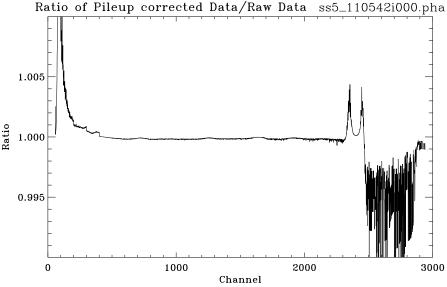
Figure 11.16: SS5 spectrum and pileup correction: Shell 6; Run ID: 110542. Upper panel shows the raw data and pileup corrected data. Dashed vertical lines indicate the X-ray lines to be used to calibrate the energy scale. Lower panel shows the ratio of pileup corrected data to the raw data.
