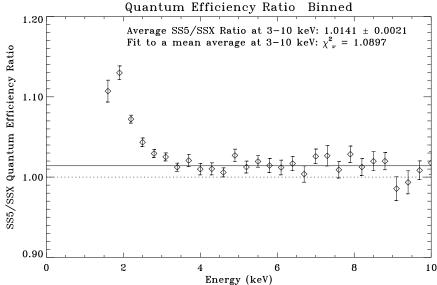
Figure 11.28: SS5/SSX quantum efficiency ratio. In the top panel, the large ratio below 2 keV is mainly due to the different ice build up on the two detectors. The bottom panel shows the ratio curve binned and fitted to a constant ratio. The solid line is the average ratio at  $3{\text -}10~{\rm keV}$ .
