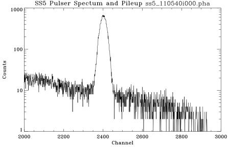
Figure 11.6: SSX and SS5 pulser spectra: Shell 3; Run ID: 110540. Counts to the right of the SSX pulser peak are the pileups from the pulser and low energy photons. Dotted vertical lines in the upper panel indicate the pulser region and four pileup bands.
