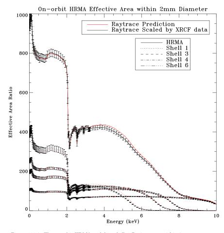
Figure 11.54: The on-orbit HRMA and four shells effective areas within 2 mm aperture. The original raytrace predictions and the calibration data scaled raytrace predictions.
