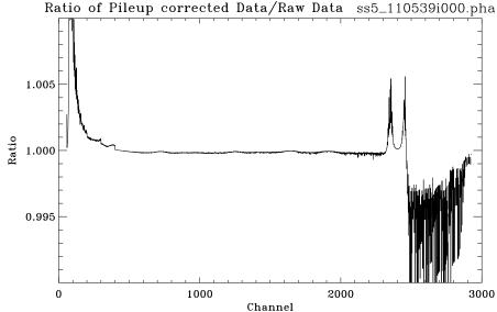
Figure 11.13: SS5 spectrum and pileup correction: Shell 1; Run ID: 110539. Upper panel shows the raw data and pileup corrected data. Dashed vertical lines indicate the X-ray lines to be used to calibrate the energy scale. Lower panel shows the ratio of pileup corrected data to the raw data.
