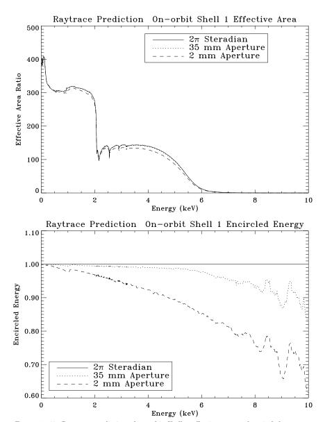
Figure 11.46: Raytrace prediction of on-orbit Shell 1 effective area and encircled energy. Top panel shows the effective area curves within 2 mm, 35 mm apertures, and  $2\pi$  steradian. Bottom panel shows the encircled energies of 2 mm and 35 mm apertures as fractions of that within  $2\pi$  steradian.
