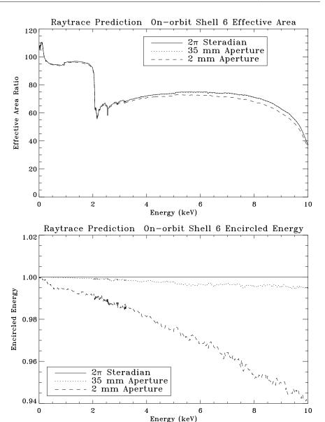
Figure 11.49: Raytrace prediction of on-orbit Shell 6 effective area and encircled energy. Top panel shows the effective area curves within 2 mm, 35 mm apertures, and  $2\pi$  steradian. Bottom panel shows the encircled energies of 2 mm and 35 mm apertures as fractions of that within  $2\pi$  steradian.
