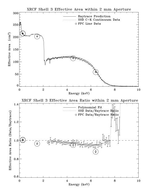
Figure 11.37: Calibration data vs. ray trace prediction. Top panel shows the XRCF Shell 3 effective area within 2 mm aperture. Bottom panel shows the effective area ratio of data/ray trace.
