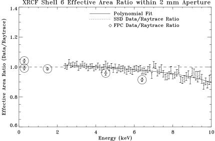
Figure 11.39: Calibration data vs. raytrace prediction. Top panel shows the XRCF Shell 6 effective area within 2 mm aperture. Bottom panel shows the effective area ratio of data/raytrace.
