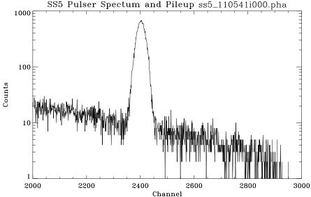
Figure 11.7: SSX and SS5 pulser spectra: Shell 4; Run ID: 110541. Counts to the right of the SSX pulser peak are mainly due to pileups from the pulser, a small amount are due to pileups from the continuum.
