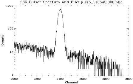
Figure 11.8: SSX and SS5 pulser spectra: Shell 6; Run ID: 110542. Counts to the right of the SSX pulser peak are mixtures of the pulser pileups and the continuum pileups.
