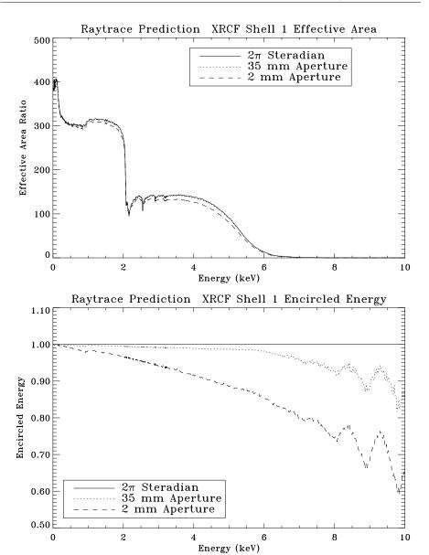
Figure 11.41: Ray trace prediction of XRCF Shell 1 effective area and encircled energy. Top panel shows the effective area curves within 2 mm, 35 mm apertures, and  $2\pi$  steradian. Bottom panel shows the encircled energies of 2 mm and 35 mm apertures as fractions of that within  $2\pi$  steradian.
