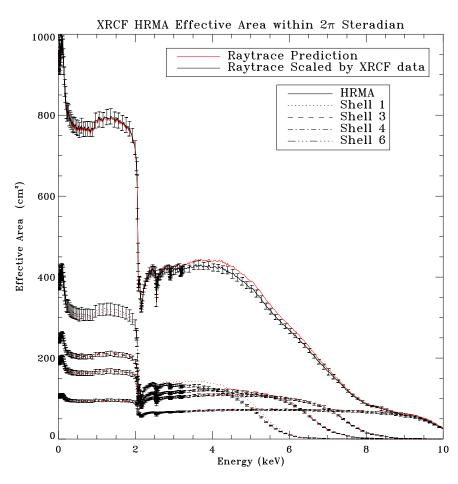
Figure 11.53: The XRCF HRMA and four shells effective areas within  $2\pi$  steradian. The original raytrace predictions and the calibration data scaled raytrace predictions.
