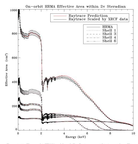
Figure 11.56: The on-orbit HRMA and four shells effective areas within  $2\pi$  steradian. The original ray trace predictions and the calibration data scaled ray trace predictions.
