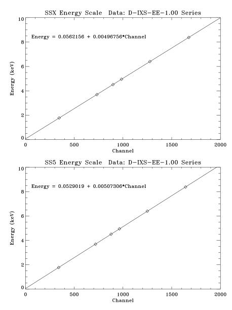
Figure 11.23: SSX and SS5 energy scales for the C-continuum effective area measurements (Phase-D), fitted with six X-ray line energies, averaged over four spectra (Run IDs: 108426, 108450, 108484, 108500).
