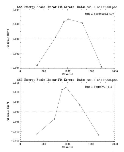
Figure 11.19: SSX and SS5 energy scale linear fit residuals for the flat field test (Phase-J).
