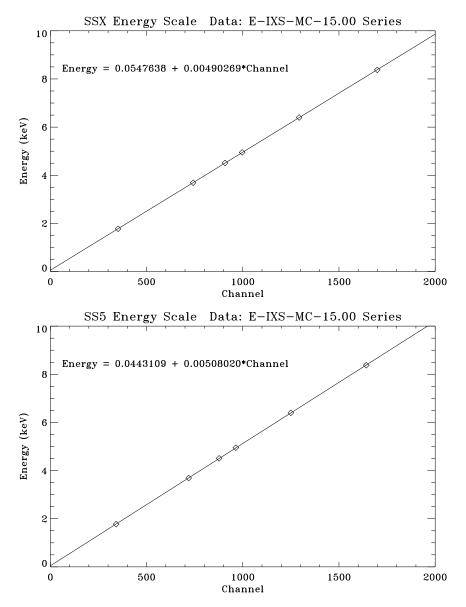
Figure 11.21: SSX and SS5 energy scales for the C-continuum effective area measurements (Phase-E), fitted with six X-ray line energies, averaged over four spectra (Run IDs 110539–110542).
