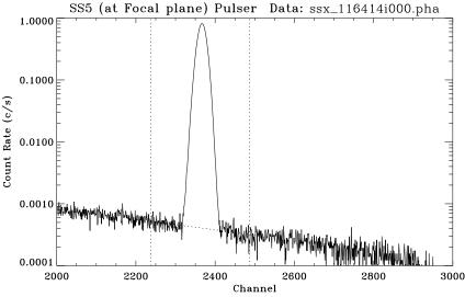
Figure 11.25: C-continuum flat field test SSX and SS5 pulser spectra. Two vertical dotted lines indicate the pulser region. A dotted line under the peak is the power law fit to the continuum. The pulser spectrum counts equal to the total counts under the pulser spectrum within the pulser region minus the total counts under the fitted power law spectrum within the pulser region.
