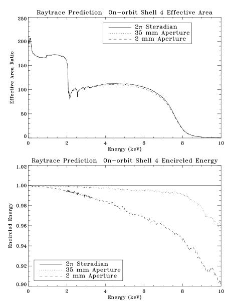
Figure 11.48: Raytrace prediction of on-orbit Shell 4 effective area and encircled energy. Top panel shows the effective area curves within 2 mm, 35 mm apertures, and  $2\pi$  steradian. Bottom panel shows the encircled energies of 2 mm and 35 mm apertures as fractions of that within  $2\pi$  steradian.
