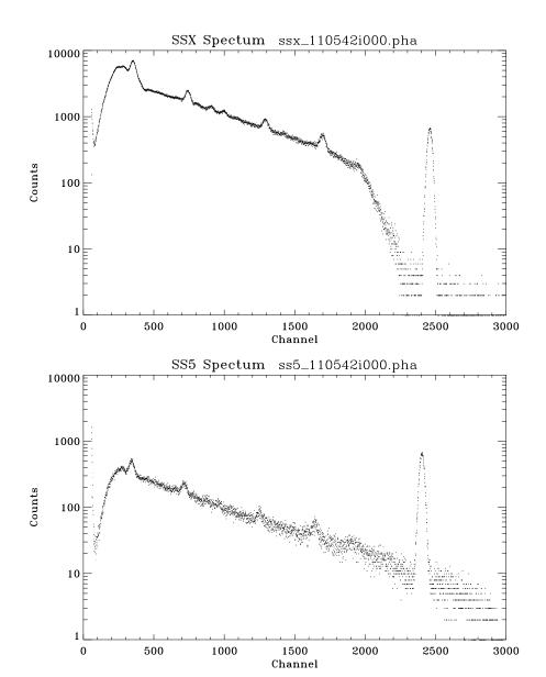
Figure 11.4: C-continuum SSX and SS5 spectra: Shell 6; Date: 970130; TRW ID: E-IXS-MC-15.004; Run ID: 110542; Aperture: 2 mm; Integration time: 1000 seconds.
