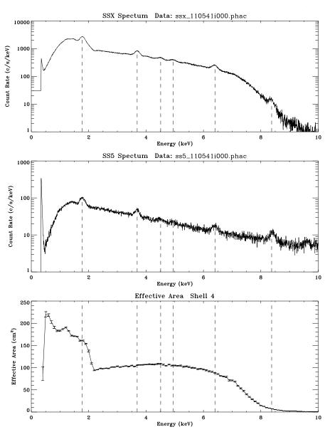
Figure 11.34: SSD C-continuum effective area measurement: Shell 4; 2 mm aperture; Run ID: 110541. Top panel is the SSX spectrum. Middle panel is the SS5 spectrum. Bottom panel is the measured effective area.
