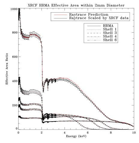
Figure 11.51: The XRCF HRMA and four shells effective areas within 2 mm aperture. The original raytrace predictions and the calibration data scaled raytrace predictions.
