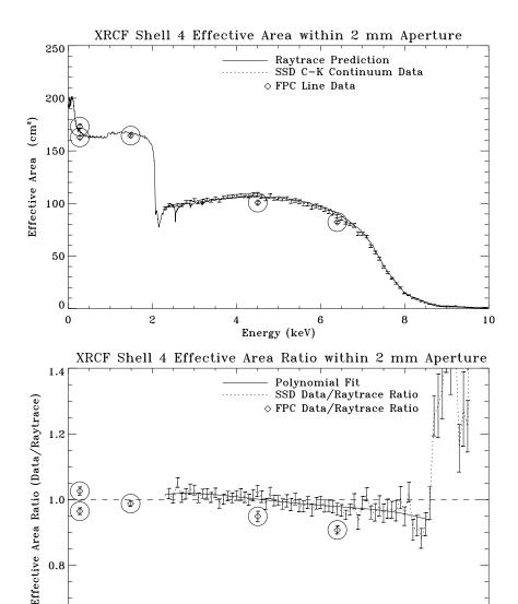
Figure 11.38: Calibration data vs. raytrace prediction. Top panel shows the XRCF Shell 4 effective area within 2 mm aperture. Bottom panel shows the effective area ratio of data/raytrace.
