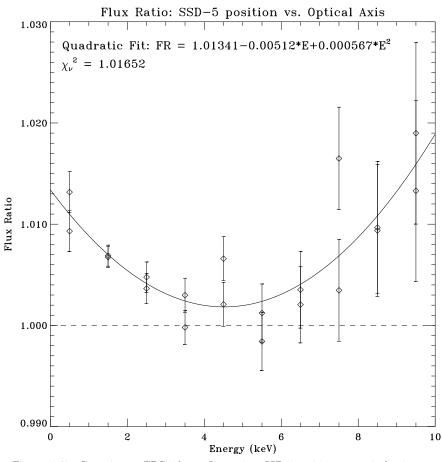
Figure 11.27: C-continuum FPC-5 beam flux ratio – SSD-5 position vs. optical axis – as a function of energy. Data are fit to a quadratic function.
