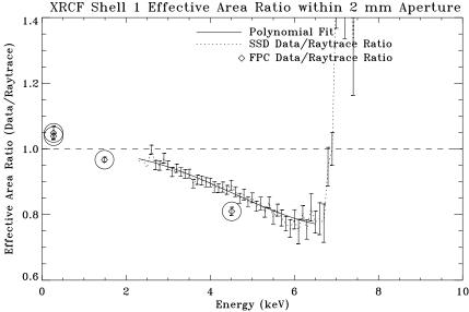
Figure 11.36: Calibration data vs. raytrace prediction. Top panel shows the XRCF Shell 1 effective area within 2 mm aperture. Bottom panel shows the effective area ratio of data/raytrace.
