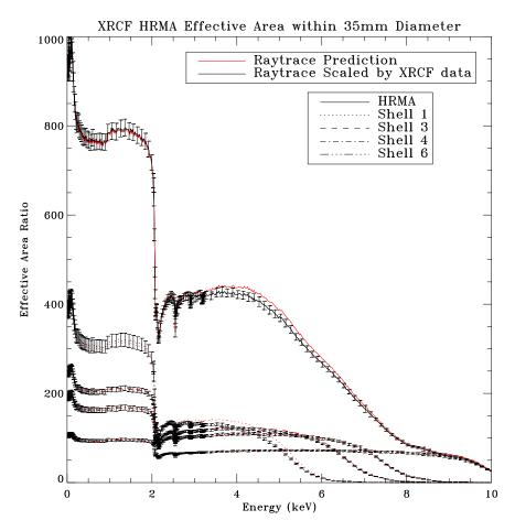
Figure 11.52: The XRCF HRMA and four shells effective areas within 35 mm aperture. The original raytrace predictions and the calibration data scaled raytrace predictions.
