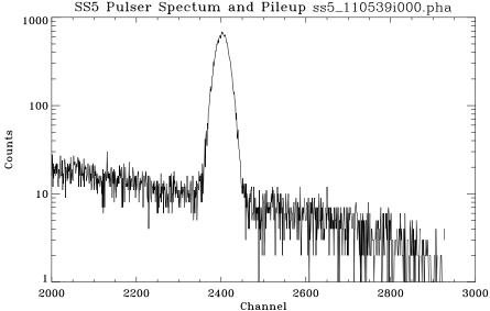
Figure 11.5: SSX and SS5 pulser spectra: Shell 1; Run ID: 110539. Counts to the right of the SSX pulser peak are the pileups from the pulser and low energy photons. Dotted vertical lines in the upper panel indicate the pulser region and four pileup bands.
