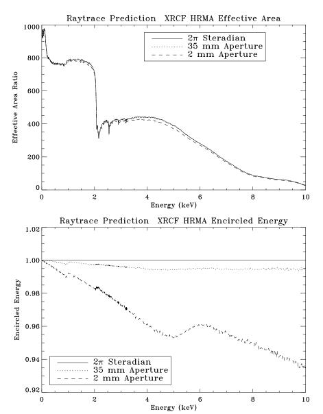
Figure 11.45: Raytrace prediction of XRCF HRMA effective area and encircled energy. Top panel shows the effective area curves within 2 mm, 35 mm apertures, and  $2\pi$  steradian. Bottom panel shows the encircled energies of 2 mm and 35 mm apertures as fractions of that within  $2\pi$  steradian.
