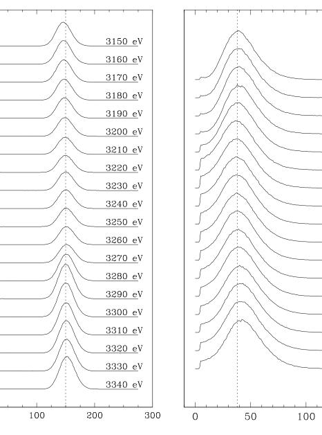
Figure 3.3: Ar-K edge scan with BESSY KMC monochromator. These data were used to measure the FPC gas opacity just below the edge. Listed energies are those requested; the true edge energy (indicated by the appearance of an escape peak and a jump in the strength of the main peak) is 3206 eV, thus calibrating the monochromator energy scale as approximately 75 eV too high. The dotted vertical line is merely to help discern relative peak positions.
