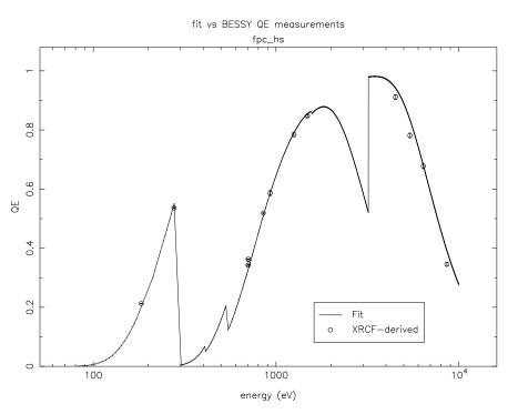
Figure 3.22: Absolute quantum efficiency for fpc\_hs from flatfield data and the fpc\_hn BESSY data (E < 1.7 keV), and derived from a theoretical SSD curve and flatfield data (E > 1.7 keV), with the fits described in the text.
