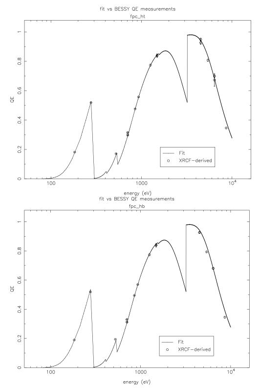
Figure 3.21: Absolute quantum efficiency for fpc\_ht (top) and fpc\_hb from flatfield data and the fpc\_hn BESSY data (E < 1.7 keV), and derived from a theoretical SSD curve and flatfield data (E > 1.7 keV), with the fits described in the text.
