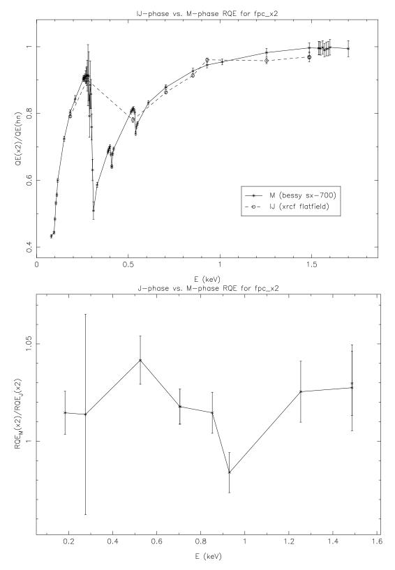
Figure 3.11: Relative quantum efficiency for  $fpc_x2$  from BESSY (phase M) and XRCF (phases I & J) flat field measurements (top) and ratio (bottom)
