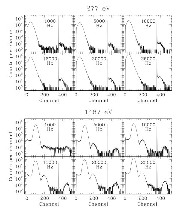
Figure 3.7: Sample spectra over a wide range of counting rate. These data can be used to measure the accuracy of deadtime-correction methods by comparing the detector counting rate with the synchrotron ring current, to study how the spectral response function varies as a function of rate, and to separate the effects of pileup and monochromator higher order contamination (since pileup is rate dependent but the fraction of higher order diffraction is not).
