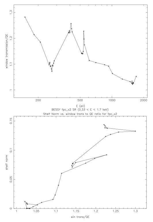
Figure 3.13: Ratio of fpc\_x2 window transmission to QE vs. energy (top) and vs. shelf norm (bottom). This suggests the QE deficit may be due to charge loss to the window.
