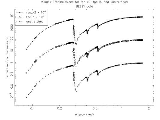
Figure 3.12: Transmission of 3 FPC windows as measured at BESSY. The windows are those of the fpc\_x2, fpc\_5, and an unstretched window. The first two curves are scaled for clarity.
