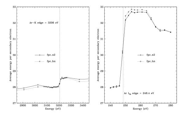
Figure 3.5: Ar-K edge work function, normalized to 28 eV below the edge. A 75-eV correction has been applied to the x-ray energies.
