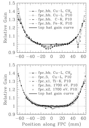
Figure 3.8: Gain scans for (top) a single FPC at several energies and with two kinds of gas, and (bottom) for several different FPCs. Vertical dotted lines mark the edges of the 99-mm blocking plates. In the top plot, the sharp dips in the P10 curves near one end are the result of an anode aging test conducted after the methane gain scan. The slight dips near the center are also from anode aging.
