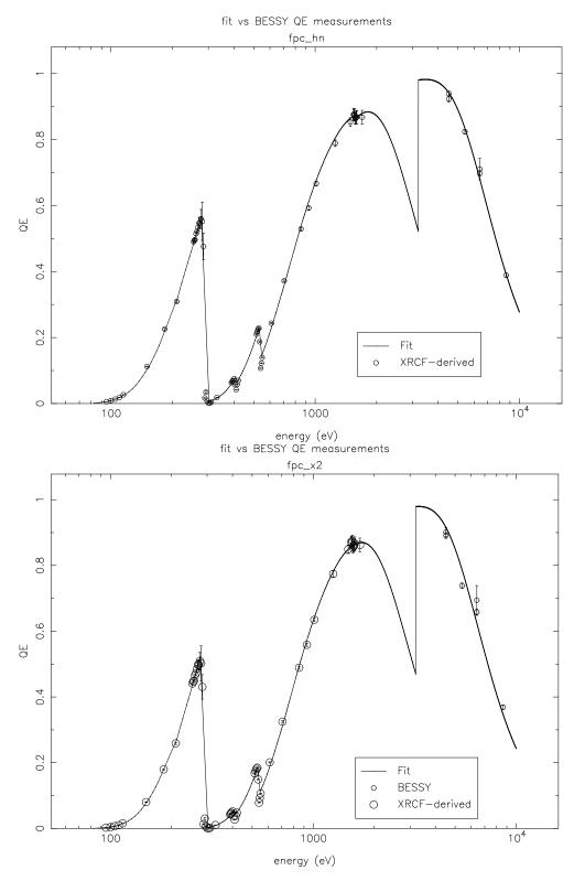
Figure 3.20: Absolute quantum efficiency for fpc\_hn (top) and fpc\_x2 from JMKmod fits to BESSY SX700 monochromator data (E < 1.7 keV) and derived from a theoretical SSD curve and flatfield data (E > 1.7 keV), with the fits described in the text.
