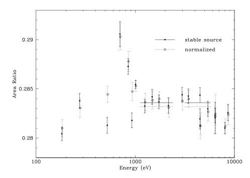
Figure 3.1: Area of fpc\_hn 36-mm aperture, relative to rectangular aperture. Ratios were calculated assuming a stable source, and by normalizing to other detectors; points are slightly separated in energy for clarity. Using results from energies where QE > 75% (indicated by horizontal lines), the unnormalized average is  $0.28360 \pm 0.00027$  and the normalized average is  $0.28317 \pm 0.00032$ . We take  $0.2835 \pm 0.0003$  as the final answer, as listed in Table 3.3.
