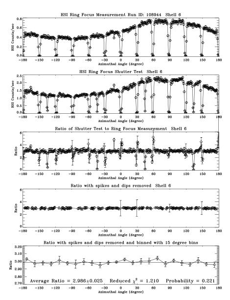
Figure 25.16: The HRMA ring focus shutter results. Shell 6
