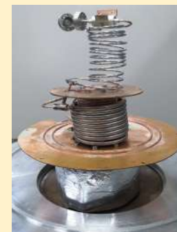
Mechanical cooler 53 mW@4 K
