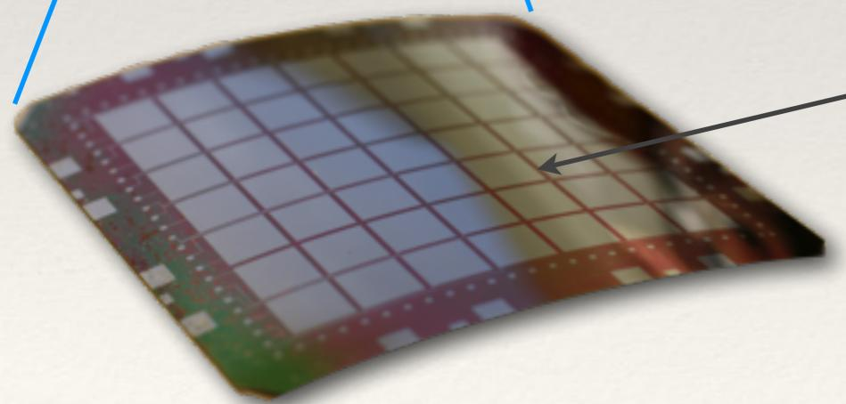
*Innovative technologies for mirror segments (MSFC, SAO, GSFC, MIT, etc.), including a possibility of in-flight adjustments with piezo cells + integrated electronics + strain gauges for in-flight feedback and control*
