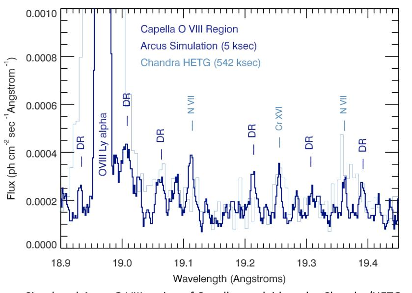
Simulated *Arcus* O VIII region of Capella overlaid on the *Chandra/HETG* spectrum. DR satellite lines of O VIII marked (DR) are identified using the AtomDB v3.0 spectral database. A 5-ks Arcus simulation will have high enough S/N to identify these lines, enabling longer observations to capture their changes in the dynamic environment of the stellar corona.
