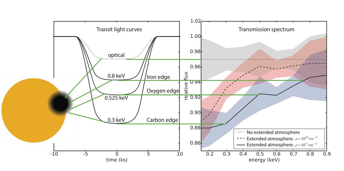
Arcus can study the density and extent of high-altitude atmospheric layers of exoplanets in close orbits by using energy-resolved transit observations sensitive to different elements. Soft X-ray photons are absorbed by low column densities in the atmosphere, causing deep transit light curves, while harder X-rays probe yet deeper layers.
