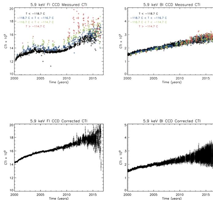
Evolution of measured CTI for the FI and BI CCDs. The colors indicate times of warmer focal plane temperature which increases CTI. The remaining structure is a combination of real radiation damage and changing particle background. Due to radioactive decay of the calibration source, it is difficult to measure CTI from a single observation in the most recent data.
