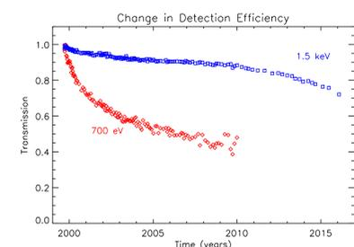
Drop in low-energy detection efficiency due to accumulating contamination on the optical blocking filter measured at 700 eV and 1.5 keV for the ACIS-S3 CCD. The 700 eV line is too weak to measure after  $\sim 2010$ .
