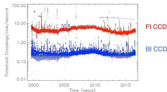
ACIS threshold crossing rate as a function of time over the entire history of Chandra. The data from each type of CCD (FI/BI) have been averaged into three minute time bins. This threshold crossing rate includes contributions both from X-ray sources in the field and from the particle background. Vertical enhancements are due to radiation events. Horizontal structures are repeated observations of bright sources (Crab and Cas-A).
