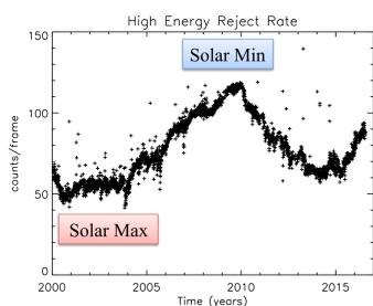
Particle background at the ACIS detector. Correlated with cosmic-ray protons ( $E > 10$  MeV); anti-correlated with the solar cycle. Many of the structures are also seen in reverse in the measured CTI.
