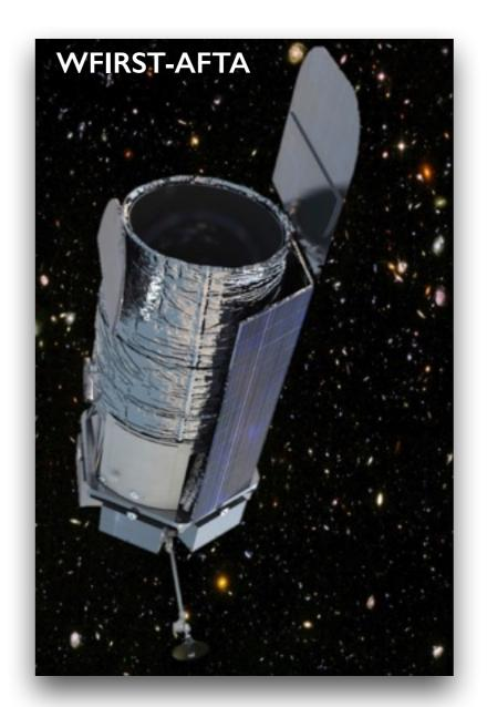
2.4 m aperture 0.28 sq.deg. FoV cosmology + exoplanets + GO program main survey: 2400 deg<sup>2</sup> to 27 mag (near-IR)
