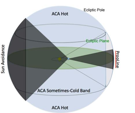
Heating and Cooling as a Function of Solar Pitch Angle
