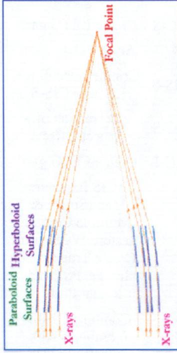
X-ray telescopes must be very different from optical telescopes. Because of their high energy, X-ray photons penetrate into a mirror in much the same way that bullets slam into a wall. Likewise, just as bullets ricochet when they hit a wall at a grazing angle, so too will X-rays ricochet off mirrors.
