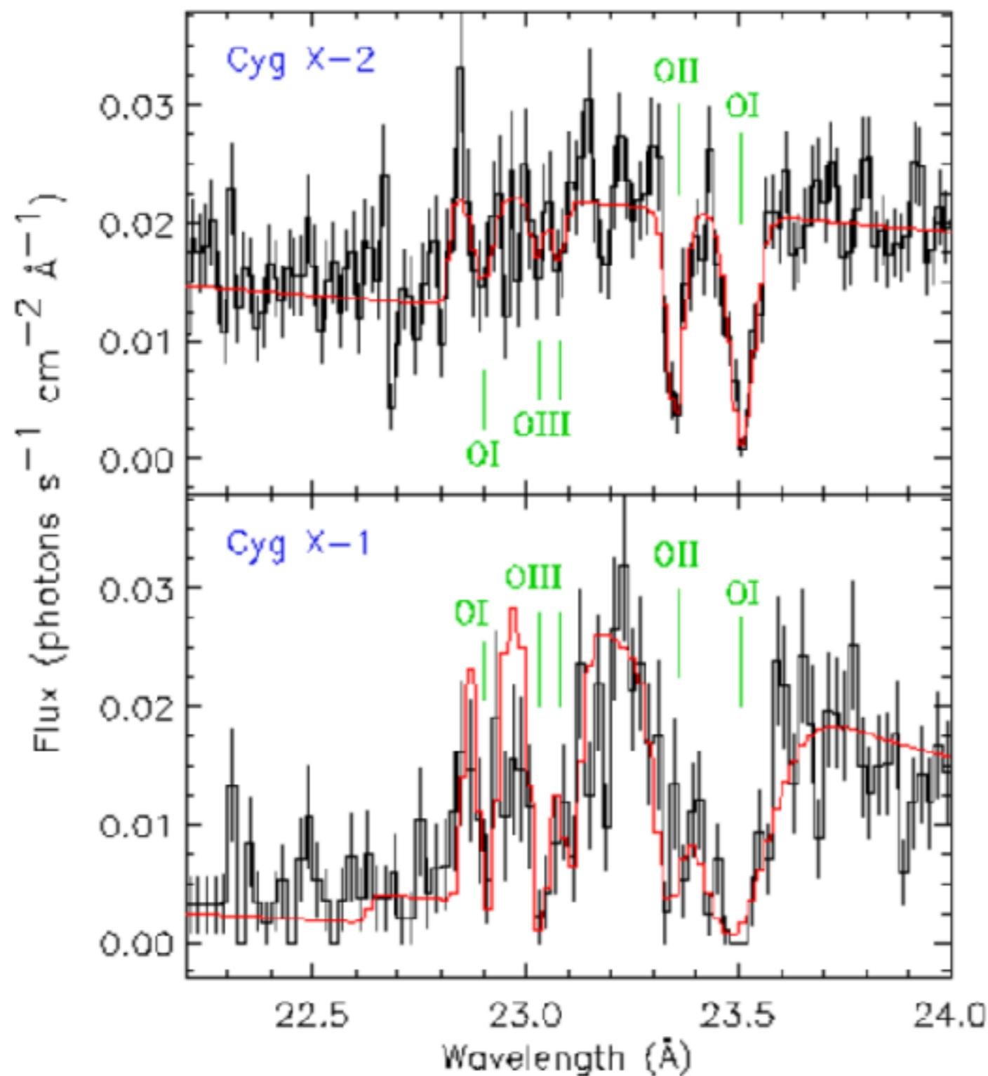
**FIGURE 11:** The bright continuum radiation from binary systems shows the imprint of the ISM along the line of sight. Absorption dips are seen in MEG spectra from neutral oxygen, O I, as well as singly and doubly ionized oxygen, O II and O III. For reference, the energy range shown is roughly 0.558 keV to 0.517 keV, left to right. From Juett, Schulz, and Chakrabarty (2004).
