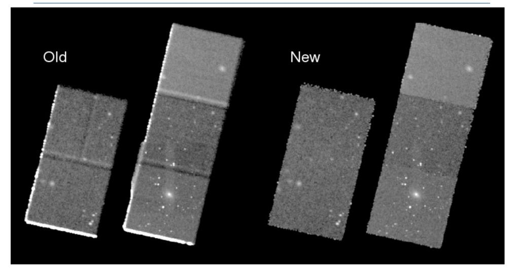
Adding four observations shows limitations of old script: obsid no 3 has a different SIM position and obsid 4 is a subarray; the new script handles the exposure maps and reprojection correctly in these cases. Avoid bad pixels at edge with thresholding CXC-SDS
