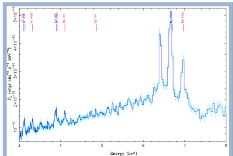
Fig. 1 — *Chandra*-HETGS spectra of the X-ray binary Cyg X-3, taken from the calibration observation that was performed simultaneously with *XMM-Newton* and *Swift*. The Fe line region is highlighted. The precision with which *Chandra*-HETGS measures the energies of these lines allows more accurate gain corrections of the other two instruments. Additionally, effective areas of all three instruments will be compared with these observations.
