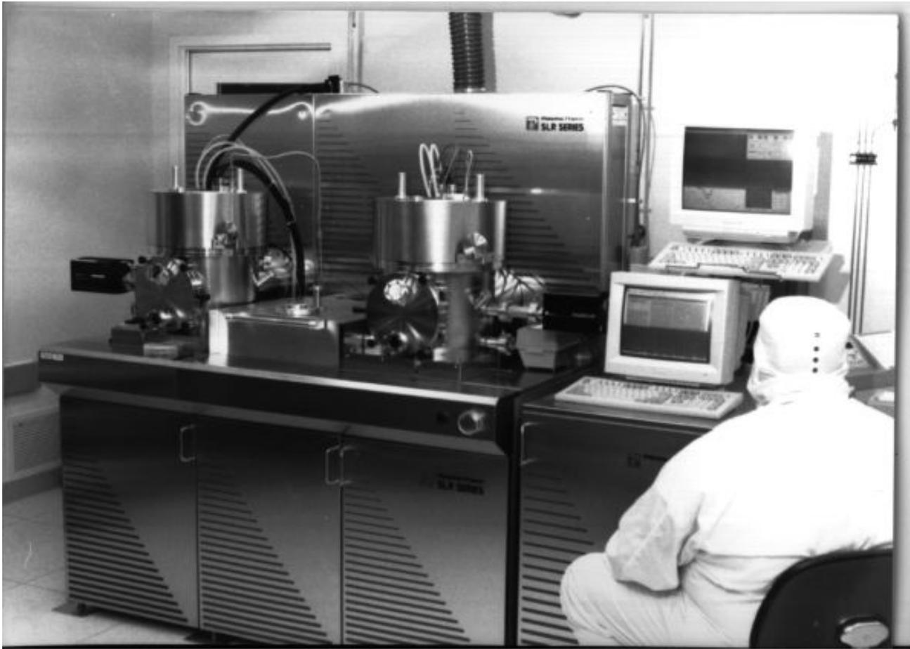
Figure 5: Reactive Ion etch plasma tool at MIT's Space nanotechnology laboratory (ca. 1995).
